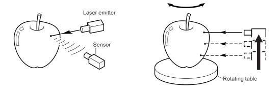
The LPX-250 has two scanning modes. Each has its own features, so you can choose the optimal scanning mode for the object to be scanned.
